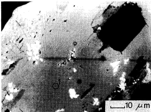
Fig. 3A. Back-scattered electron images (BEI) of homogeneous allanite with thorite grains (white spots) from porphyroblastic granitoid (see Tab. 2, No. 1 analysis, Mecsek Mts.: Mórágý).
